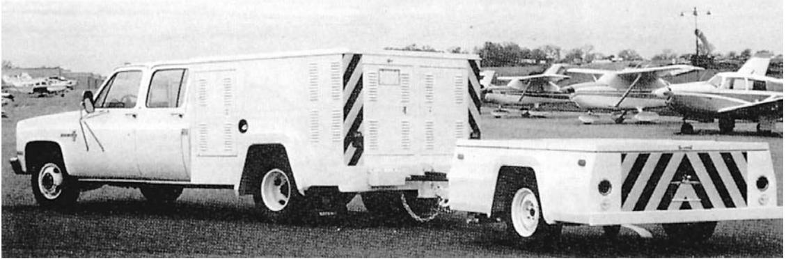
Figure 21.12 Locked-Wheel Skid Trailer
