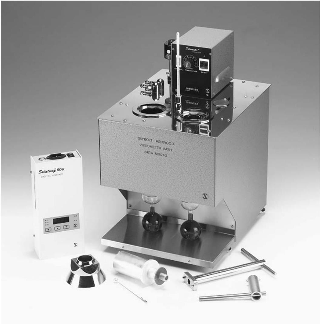
Figure 18.2 Saybolt Furol Viscometer
