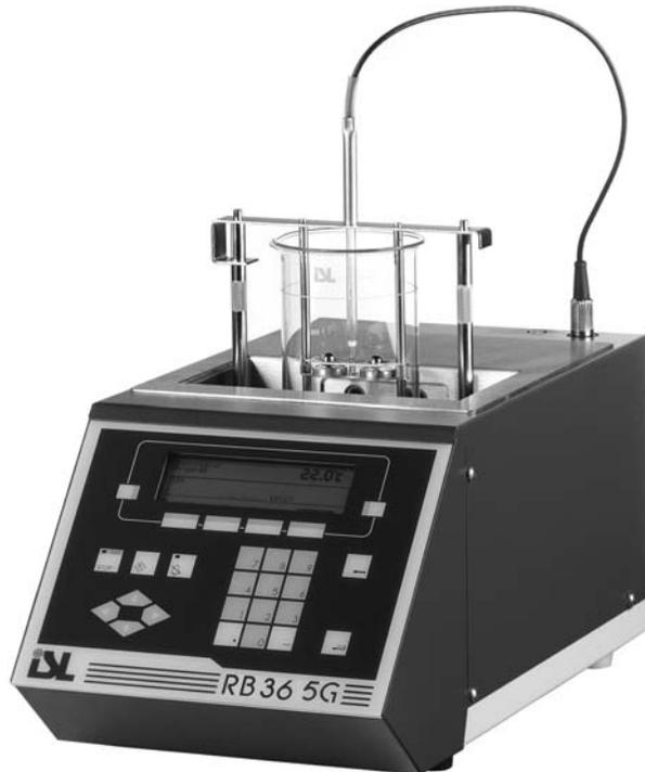
**Figure 18.6** The RB36 5G Automated Ring-and-Ball Tester
