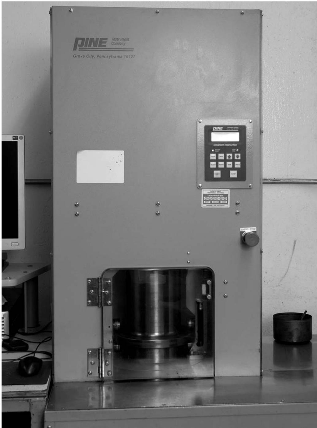
Figure 18.17 Superpave Gyratory Compactors
