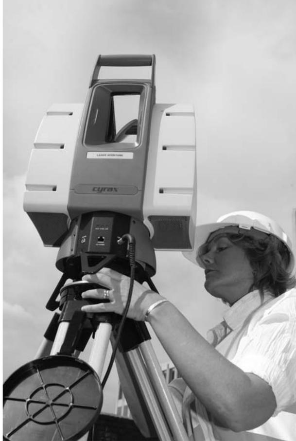
**Figure 14.14** Leica HDS3000 High Density Scanner
