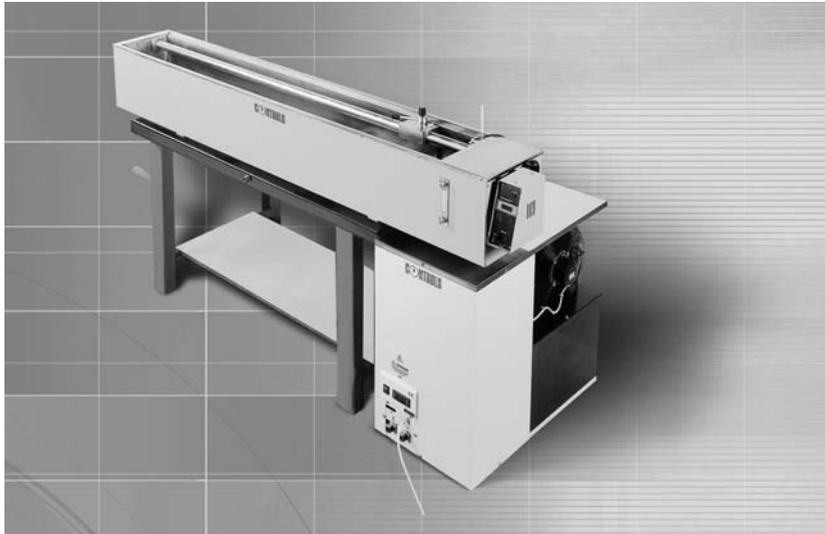
Figure 18.9 Apparatus for Ductility Test
