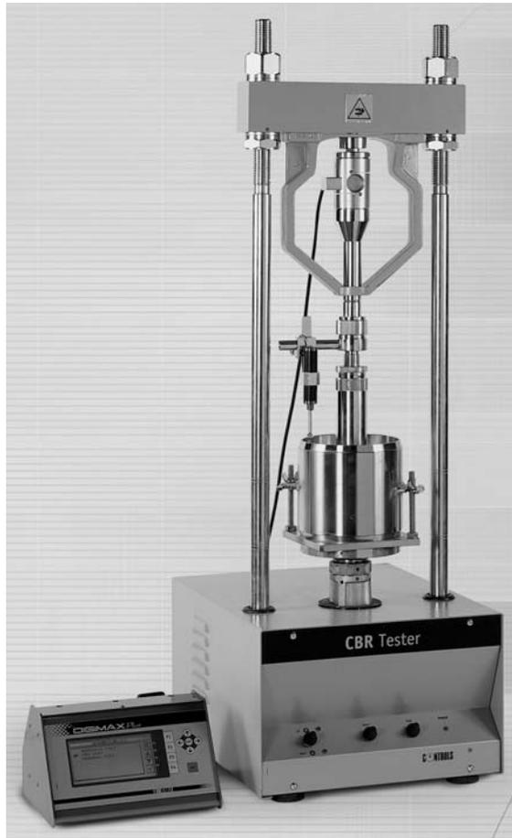
Figure 17.17 CBR Testing Equipment
