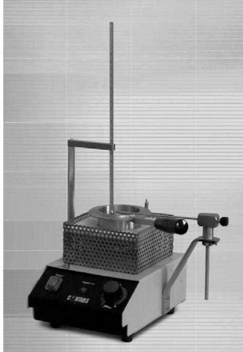
**Figure 18.10** Apparatus for Cleveland Open-Cup Test
