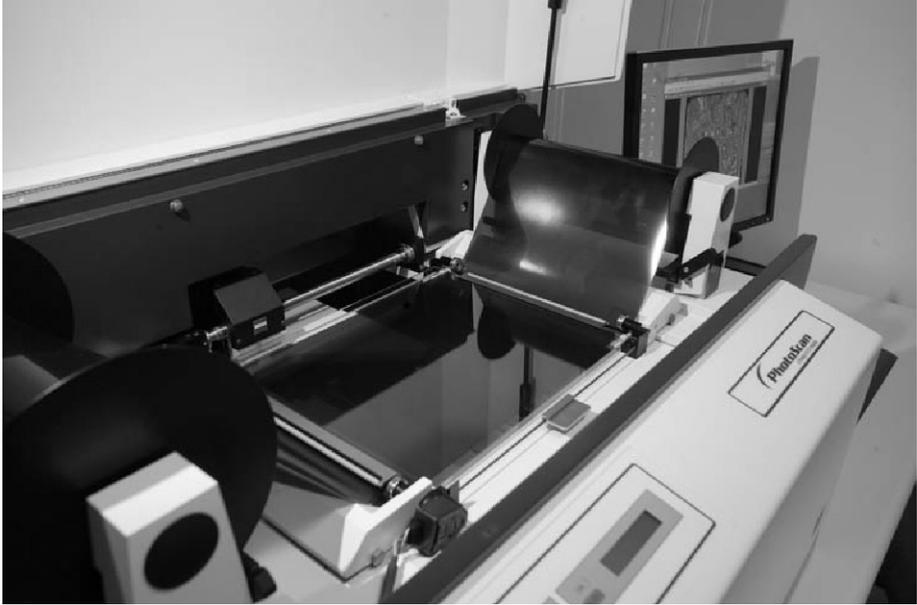
**Figure 14.9** Photostan Roll-Film Photogrammetric Scanning System
